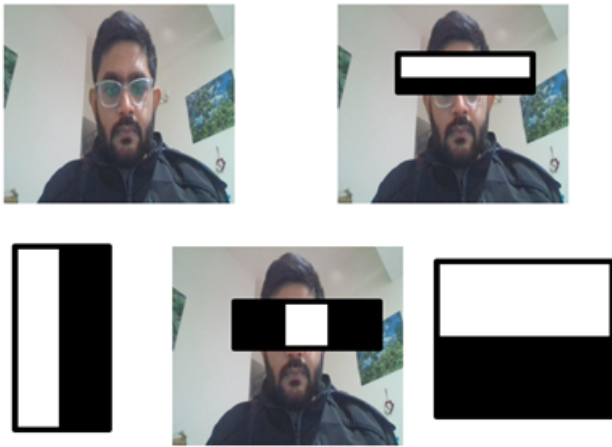
FIGURE 4: Face Identification through HAAR cascade model [40]
