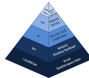
Figure 4. Application classification for OWC depending on transmission distance
